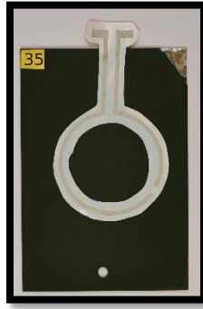
Figure 1: This sensor is attached to a carbon steel panel coated with full CARC system. The two sensor electrodes are silver-silver-chloride ink screenprinted on a polyimides substrate.
