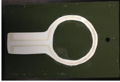
Figure 1: The photograph of the electrochemical impedance (EIS)-based sensor with screen-printed Ag/AgCl counter and reference electrodes adhered to a coated Army test panel.
