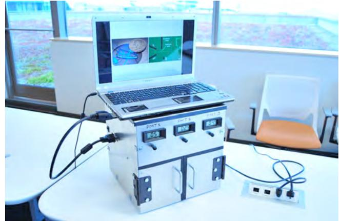
Figure 2: Phase I prototype of a fully functional flow cytometer with customizable PMT voltages (LCDs). The heart of the flow cytometer, microfluidic 3D cell focusing device, is installed inside the upper compartment of the prototype.
