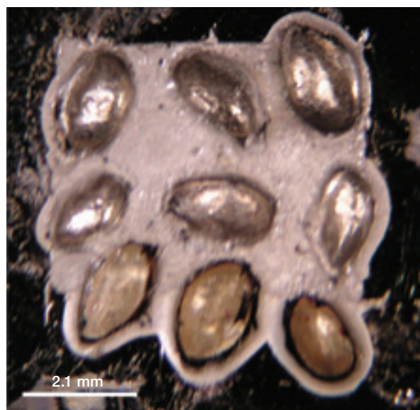
Optical image of the underside of a 3 x 3 array of blowfly corneas after coating, electroforming and removing some of the corneas. In this photograph, the corneas have been removed from the upper two rows to reveal the negative, but they have been left in place in the bottom row.
