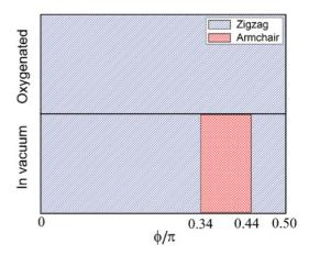
FIG. 6. (Color online) A map of the preferred fracture paths in the plane of chemical condition and crack-tip mode mixity  $\phi$ . The preferred fracture paths are shaded differently (slashed for zigzag direction, and cross-hatched for armchair).
