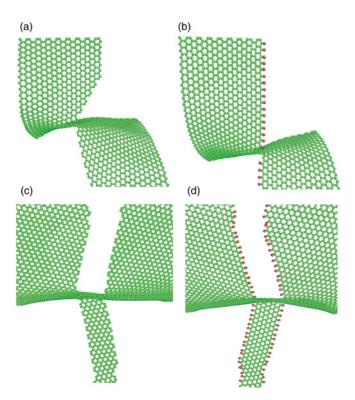
FIG. 2. (Color online) Fracture paths in graphene determined by direct MD simulations, where red dots represent oxygens and green dots represent carbons. Tearing in vacuum or in the presence of hydrogens (not shown) causes notch extension along the armchair direction (a), but along the zigzag direction in the presence of oxygens (b). GNRs with edge orientations [(c) and (d)] corresponding to different chemical additives are produced by tearing off a graphene sheet with two initial notches.
