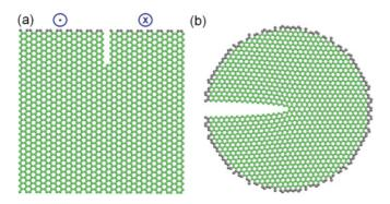
FIG. 1. (Color online) The simulation models. (a) The finite-sized crack model. Edge atoms in gray are fixed and subjected to out-of-plane pulling with directions denoted by circled dot (outward, for the edge atoms on the left) and circled cross (inward, for the edge atoms on the right), respectively. (b) The semi-infinite crack model. Atoms at the outer layer (in gray) are held fixed, while the remainder of the atoms are free.
