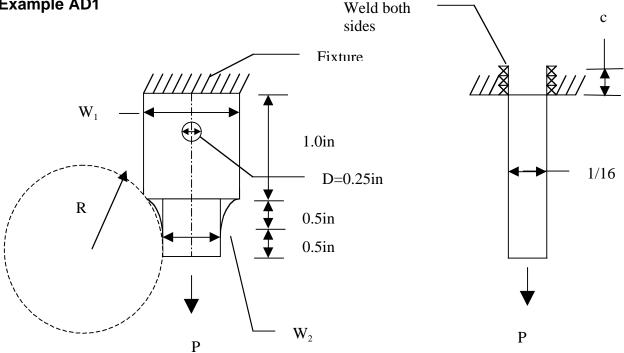
Design the A-36 steel hanging bracket so that it will carry a load of 1000 lb and not generate significant stresses in the transition from region of load application to location of the 1/4 inch diameter hole. The bracket has a thickness of 1/16 inch and is welded on both sides a depth c into the fixture. The bracket cannot deform while loaded more than 0.005 in. Use a factor of safety of 1.3.
