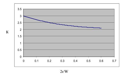
Here r is the radius of the hole and W is the width of the plate, not the thickness. It is interesting to note that the maximum K is 3.0, hence in the absence of data, one can design conservatively using this value.
